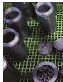
Phase 5 Positioning of the components over the grill of the oil tank. The oil is used to saturate the surface in order to avoid possible future corrosion of the components.
