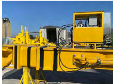
Stabilization systems for wind turbines' foundations with special cylinders and power packs suitable for marine environment.
