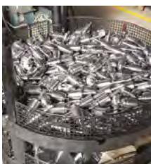
Phase 3 Positioning of the components for the NITREG process in the furnace.
