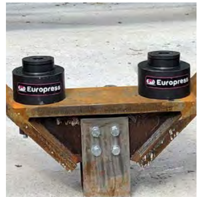
Special cylinders for high temperatures, fitted on resistance verification equipment to test flameproof concrete tunnel segments
