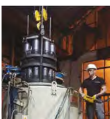
Phase 4 Positioning of the components inside the oven for the NITREG process.
