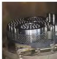
Phase 3 Positioning of the components for the NITREG process in the furnace.
